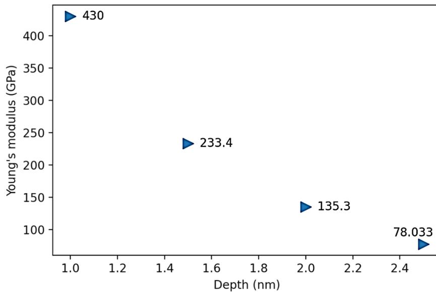
**Fig. 11: Variation of young's modulus for different depth using Euler's equation**
