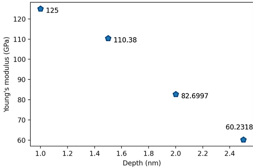
**Fig. 12: Variation of young's modulus for different depth using Modified Euler's equation**
