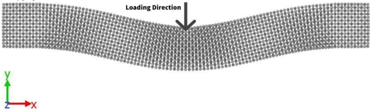
**Fig. 2: Beam Bending under Uniaxial Central Load**
