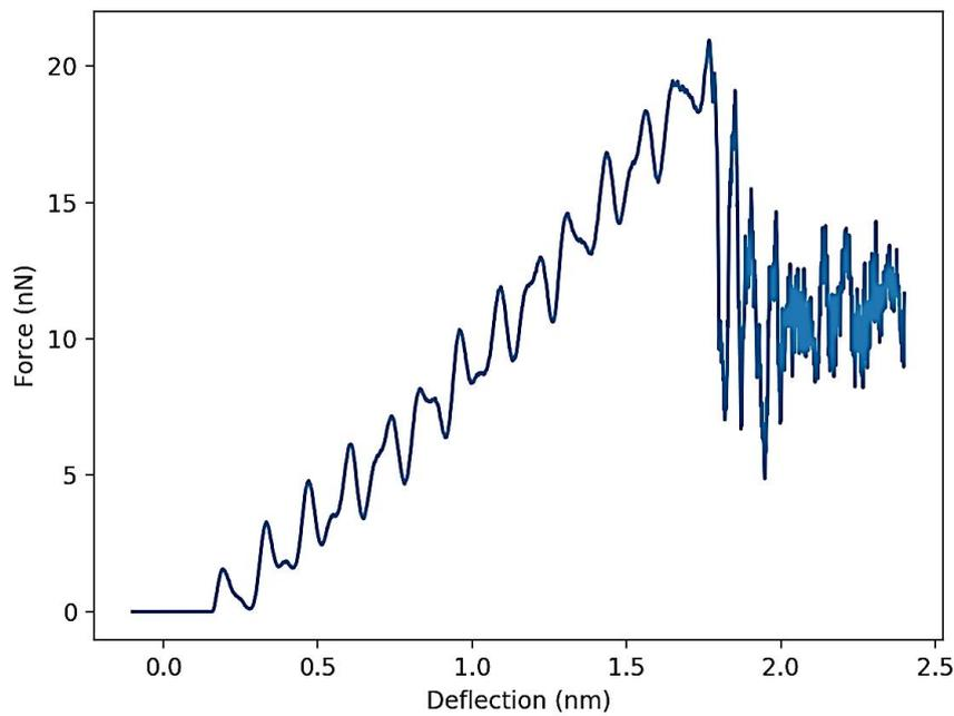
**Fig. 3: Bending result of a Cu NW (20 nm X 2.5 nm X 2.5 nm) under 1m/s loading rate at 0.01k temperature**
