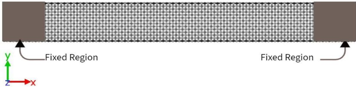
**Fig. 1: Three Point Bending Model of Cu NW for MD simulation**
