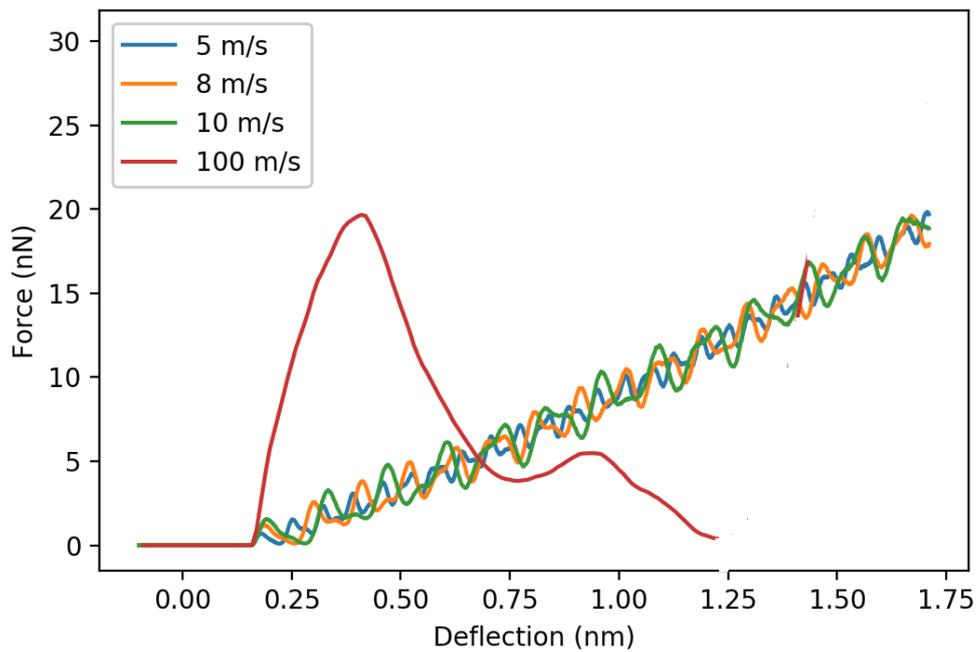
**Fig. 6: F-d curve for different loading rate**
