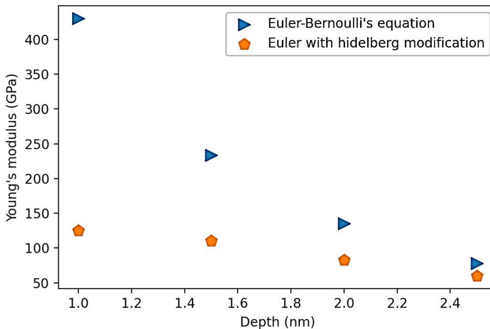
**Fig. 13: Comparisitional analysis of young's modulus variation due to different depth using Euler and Modified Euler equation**
