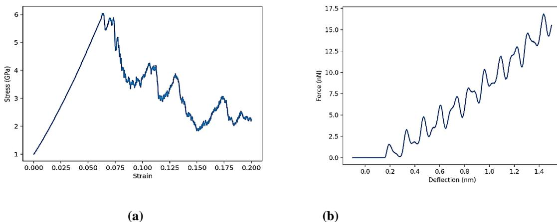
**Fig. 4: (a) Tensile result of a Cu NW (20 nm X 2.5 nm X 2.5 nm) at 0.01k temperature (b) Bending result of a Cu NW (20 nm X 2.5 nm X 2.5 nm) at 0.01k temperature**
