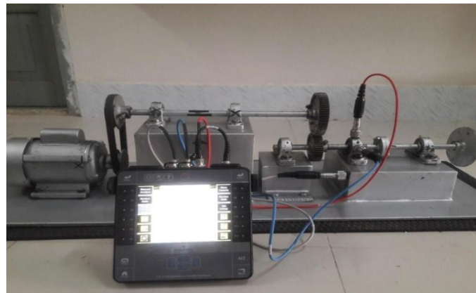
Fig.5: Experimental setup with vibration analyzer.
