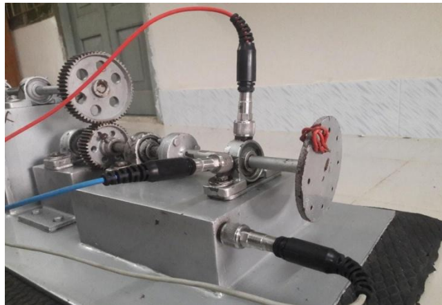
Fig 7.20: Balancing mass added in the rotating load.
